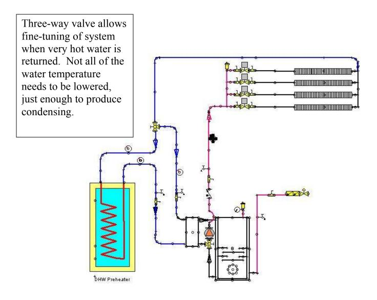
This concept could be used with any combination of heat emitters. The object here with baseboard is to lower the return water sufficiently enough to promote condensing. The concept could also encompass HRV preheating of air, or other devices to remove heat from the return water.
