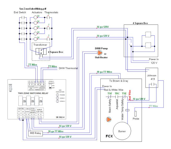
This sample controls 5 zones using 3 thermostats.
