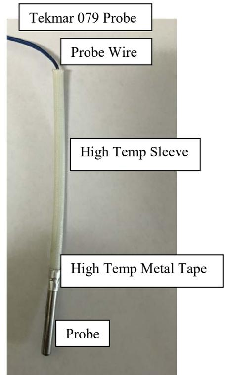
Note: Tekmar Boiler Temperature Probe needs to be a 10,000 ohm type 2, and no larger than about 3/16" in diameter. A Tekmar 079 will work. If using the Johnson 419 the 1/4" probe will work only by drilling out well to 9/32. A 12" long bit is needed if not disassembled.
