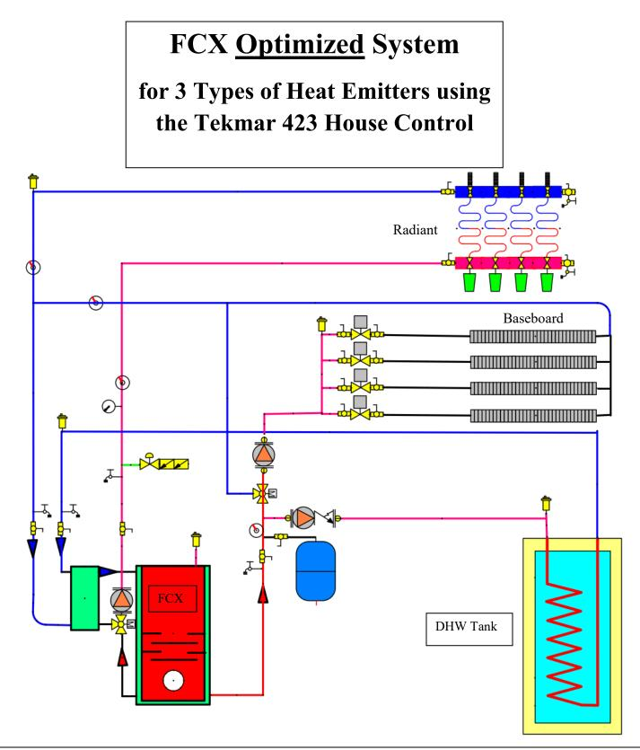
This schematic shows how to optimally plumb a home that contains both Radiant and Baseboard emitters, with DHW. Here the Tekmar 423 house control is modulating 2 motorized mixing valves to produce 2 water temperatures and is simultaneously setting the DHW temperature by controlling the boiler temperature
