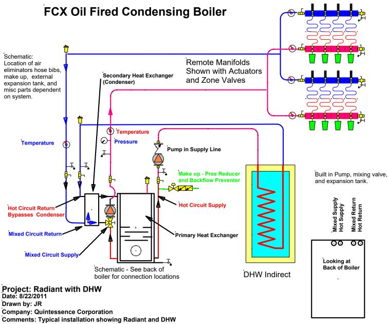
circuits, with FCX boiler schematic. Component placement will vary.
