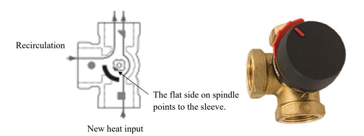
The preferred position is to have the indicator pointing up when the sleeve is left (blocking the recirculation) and the rooster tail up. So when the red mark is up pointing to the top this is full hot supply. Turning it 1/4 turn counter clockwise makes it full recirculation (no hot water added). The rooster tail has the correct stops in this position.
